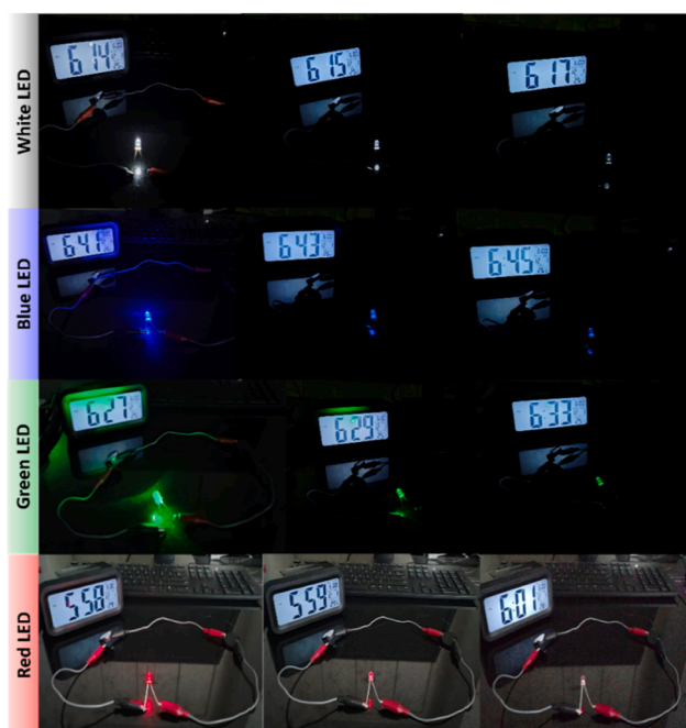
Fig. 14. The practical application of SSSC coin cell for glowing various colour LED light illumination under room temperature condition (Temperature: 32^\circ\text{C} ; Relative Humidity: 40 %).
